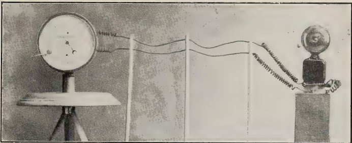
Fig. 75. Bolton alarm thermometers, showing thermometer, wires, bell and battery.
